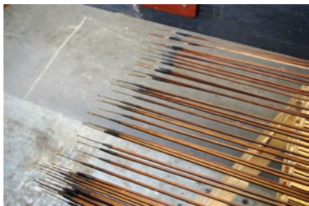
Newly restored tracker rods with threaded wire terminals.
