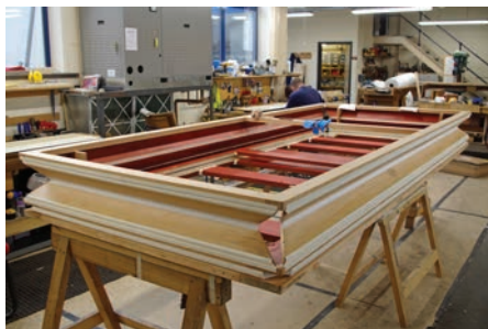
One half of the refurbished air reservoir showing new leather hinges. The red is a traditional coating of glue solution used to seal the timber members.
